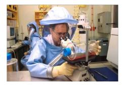
For BSL-4 labs, which require the highest safety standards, lab personnel should work in fully encapsulated suits. The positive pressure suit shown here is decontaminated using a chemical shower. (*Photo courtesy of Tony Della-Porta.*)
